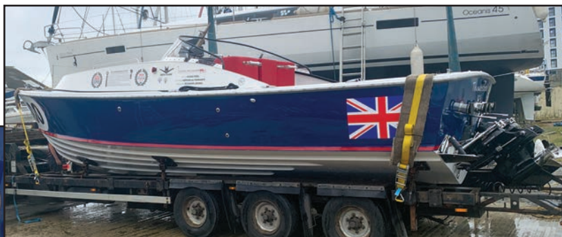
Below and right: Thunderstreak's MerCruiser sterndrives and extended Lenco trim tabs, gearbox cooling-showers. With its many championship decals, the boat is shown en route to win the Cornish 100 race.
