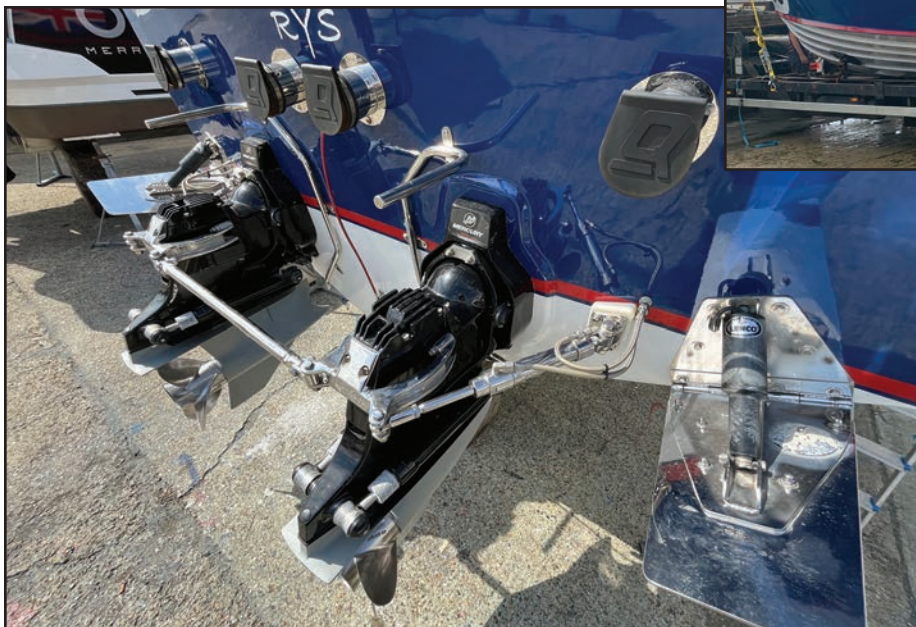
Below and right: Thunderstreak's MerCruiser sterndrives and extended Lenco trim tabs, gearbox cooling-showers. With its many championship decals, the boat is shown en route to win the Cornish 100 race.
