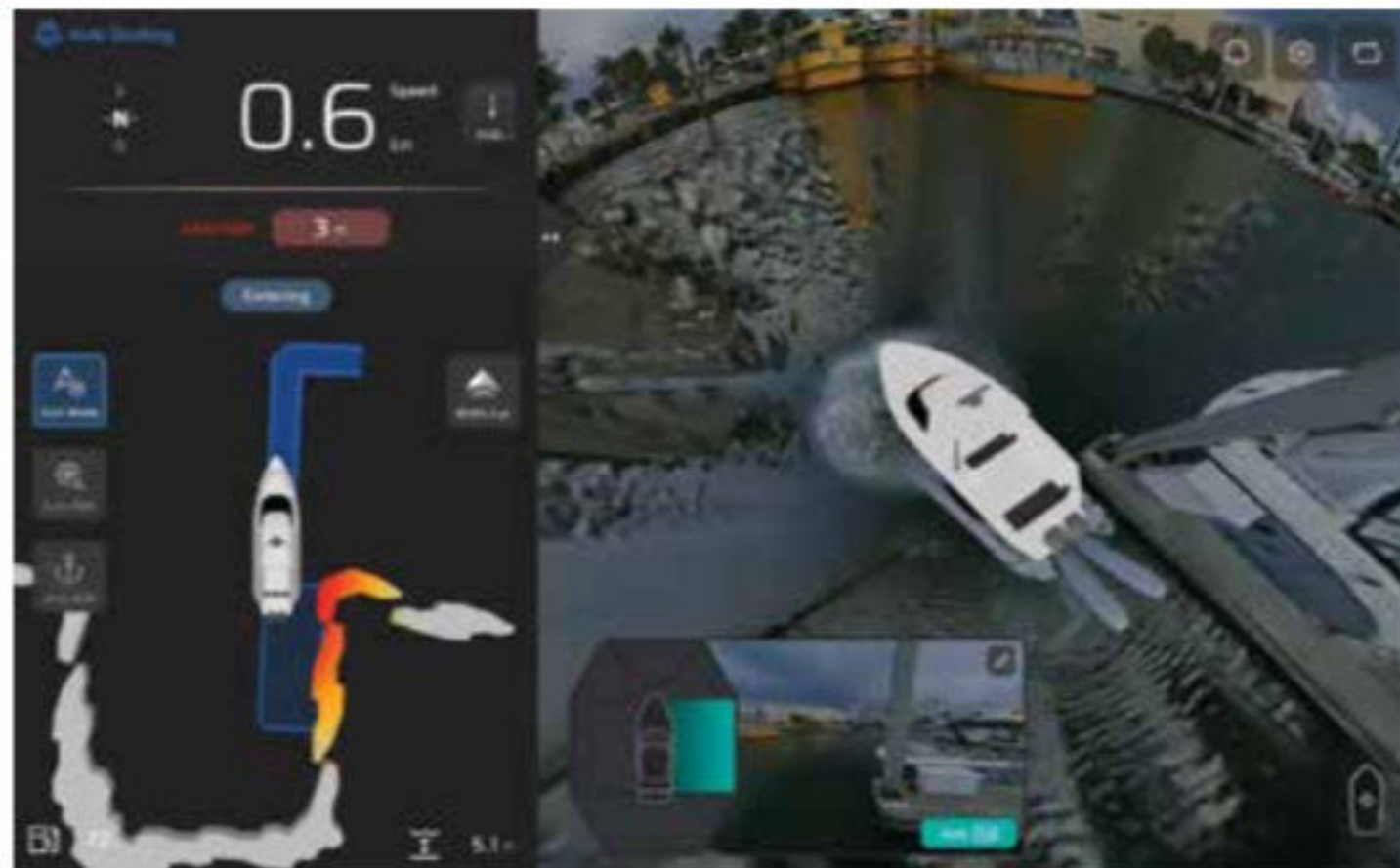
BACKING IN Avikus' docking technology utilizes six cameras to create a 360-degree view, while also using AI to recognize obstacles and distances.
