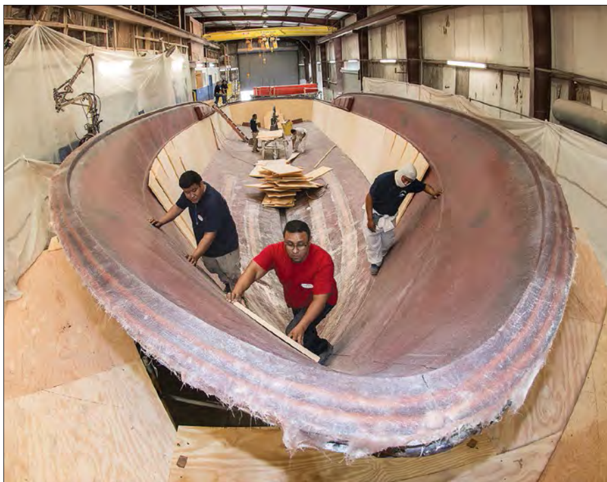
Crews build the foam-cored infused FRP hulls of the R-76 in Bradenton.
