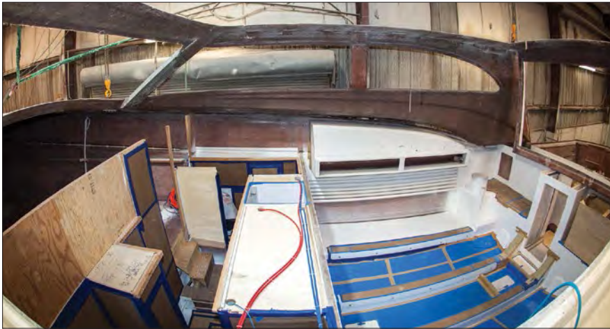
Interior components going into an R-76 in Bradenton include the spacious white-painted engine room to the right, and the crew quarters fitted below the saloon sole on the left.
