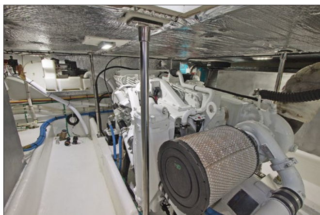
Left —The reconfigured engine room houses a remanufactured 6CTA 8.3-liter 430-hp Cummins diesel. Right —The battery bank was relocated farther aft and connected to an upgraded charging system. Note the new sound insulation lining the engine room.
