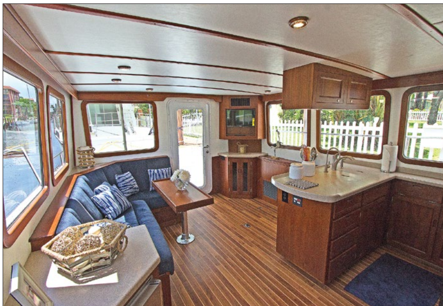
New windows, teak trim, vinyl sole, and countertops grace the galley and aft saloon.
