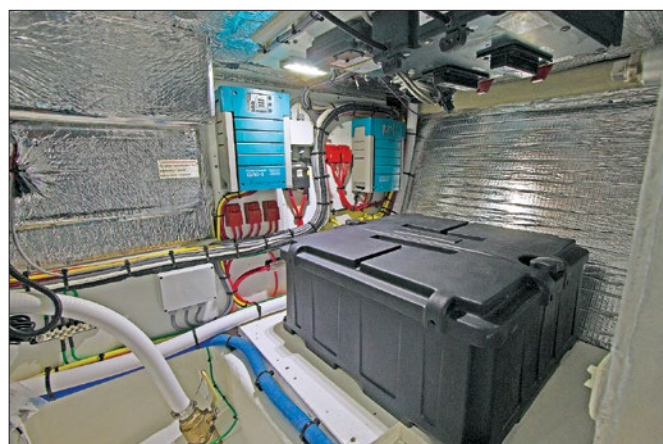
Left —The reconfigured engine room houses a remanufactured 6CTA 8.3-liter 430-hp Cummins diesel. Right —The battery bank was relocated farther aft and connected to an upgraded charging system. Note the new sound insulation lining the engine room.
