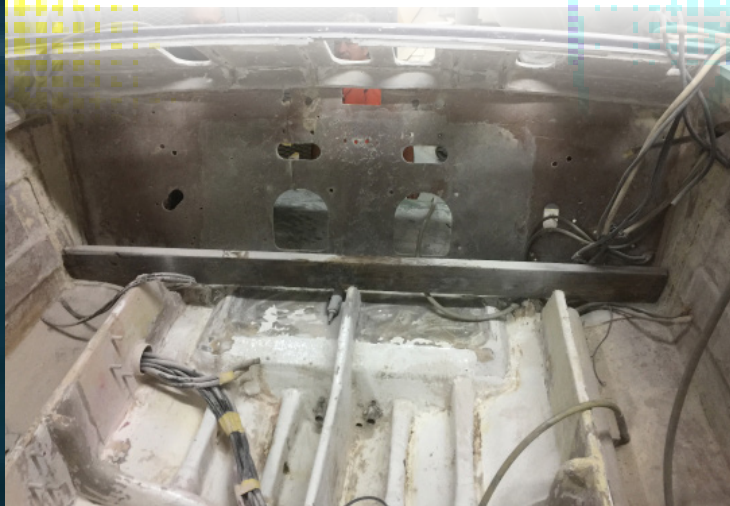
Left: Years of neglect and stagnant salt water left stringers, fuel tanks and fiberglass on the Apache in a sorry state, but TNT Custom Marine worked hard to get everything back into shipshape. The entire dashboard, helm and engine compartment was gutted and refurbished. Guardardo Marine worked tirelessly on restoring fiberglass and applying new paint.
