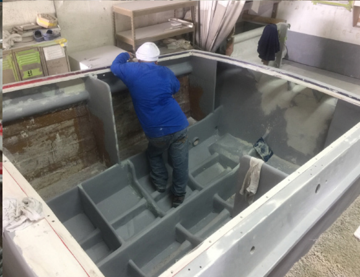
Left: Years of neglect and stagnant salt water left stringers, fuel tanks and fiberglass on the Apache in a sorry state, but TNT Custom Marine worked hard to get everything back into shipshape. The entire dashboard, helm and engine compartment was gutted and refurbished. Guardardo Marine worked tirelessly on restoring fiberglass and applying new paint.
