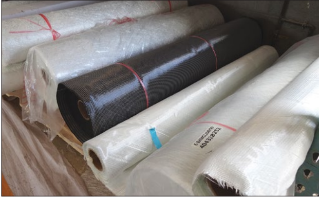
Above —Laminate materials in Barker's shop include various weights and weaves of E-glass, Kevlar, and carbon fiber. Right —In the shop a builder finishes a hand-laid console unit.
