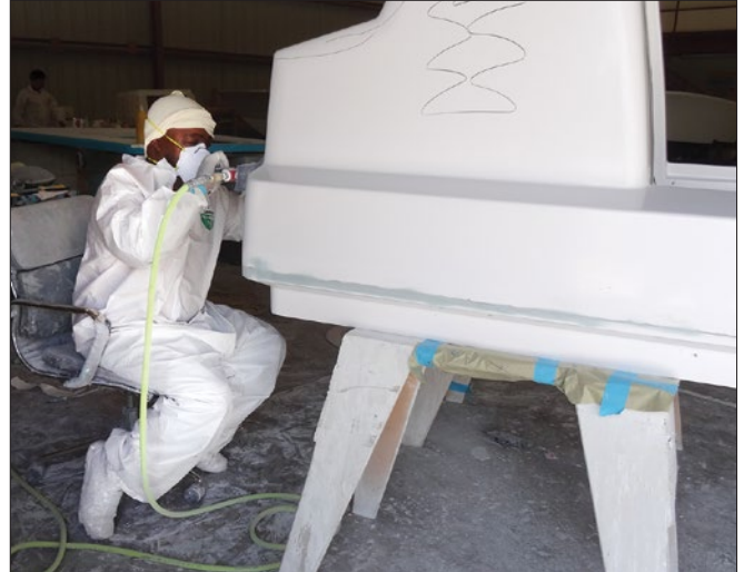
Above —Laminate materials in Barker's shop include various weights and weaves of E-glass, Kevlar, and carbon fiber. Right —In the shop a builder finishes a hand-laid console unit.
