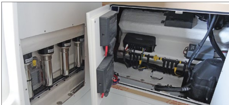
Left —Shown here, electrical harnesses made by Marine Digital Integrators in Stuart are some of the systems components Barker subs out to a selection of the many specialized shops in South Florida. Right —Hatches are lined with foam flooring material that acts as a gasket to seal out water and prevent hatch and door rattles.
