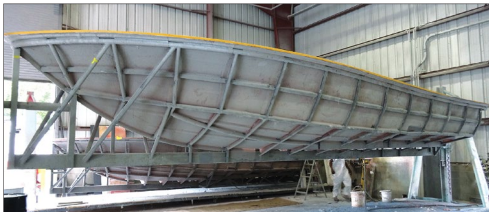
Neighboring Marine Concepts built the sophisticated tooling necessary for resin infusion hull construction, which Barker favors.
