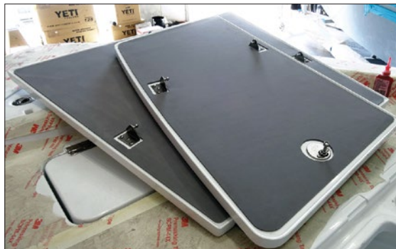
Left —Shown here, electrical harnesses made by Marine Digital Integrators in Stuart are some of the systems components Barker subs out to a selection of the many specialized shops in South Florida. Right —Hatches are lined with foam flooring material that acts as a gasket to seal out water and prevent hatch and door rattles.
