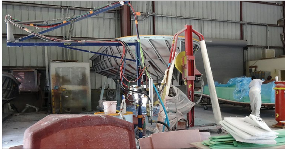
In the lamination shop, hull and deck tooling are readied for infusion. In the foreground are molds for smaller hand-laid parts and components.
